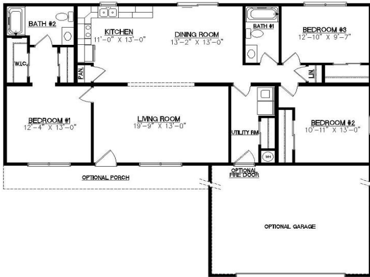
First Floor (w/ Crawl Space)
